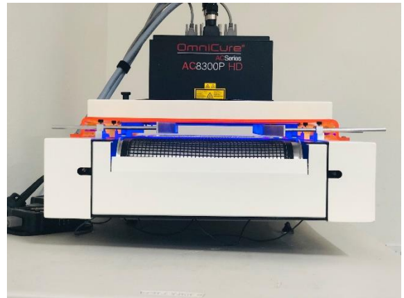
48" x 12" UV Curing Conveyor shown with Dual AC8 LED Heads, Acrylic UV Safety Light Shields and Guide Rails
